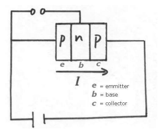
A small AC current in the emmitter-base circuit produces a large current flow in the emmitter-collection circuit that is proportional to the AC current in the emmitter-base circuit. This is a transistor amplifier.
