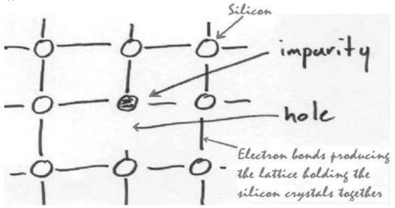
• In n-type semiconductors there are more negative charge carriers than positive holes. Elements, such as arsenic and phosphorus (5 valence electrons), are used as doping agents with silicon to produce n-type semiconductors.
