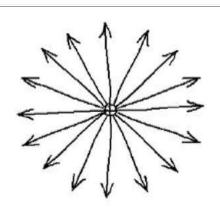
The number of the lines drawn to represent a field at any point indicates the electric field strength at that point. The stronger the field, the more lines are drawn in a given space.
