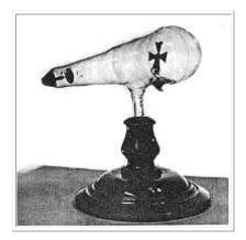
• Plucker made an anode into a Maltese cross, and this produced a shadow in the glow at the end of the tube. This showed that the cathode rays traveled in straight lines.
