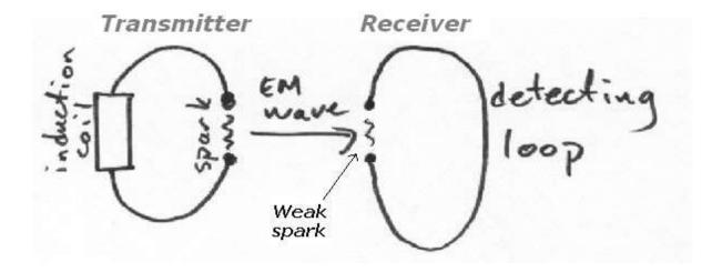
Hertz was able to calculate the velocity of the waves by reflecting the generated waves off a metal sheet and measuring the wavelength of the standing wave set up by interference. Substituting this wavelength and the known frequency of the wave generator into the general wave equation, v = ? x f, Hertz calculated the wave speed at  $3 \times 10^8 \text{ ms}^{-1}$ , very close to the values for the speed of light earlier estimated by Maxwell and measured by Fizeau.
