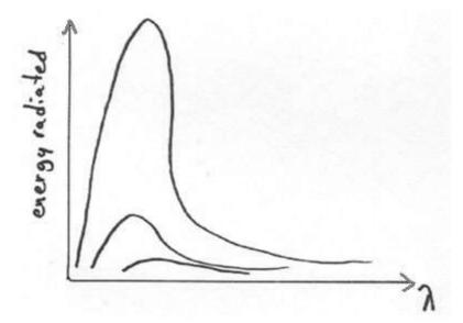
• Planck's explanation for the observations involved the radical idea that energy could only be radiated or absorbed in small discrete amounts, later called quanta, now identified as photons. The size of each quantum of energy is characteristic of the frequency of light emitted.
