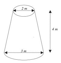
Volume of large cone (h=12m, d=3m) subtract the volume of small cone (h=8m, d=2m).
