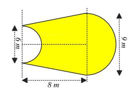
The shaded area is the area of the trapezium in the centre add the area of the large semi-circle subtract the area of the small semicircle. The trapezium has parallel side lengths 6m and 9m separated by a
